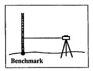
Fig. 6-1 Starting the line levelling
