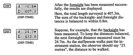
You can test the distance value at any time by pressing the  $\boxed{\text{INP/D}}$  key (see section 8.4.2).
