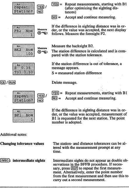
For the NA3003 in BFFB mode, intermediate sights are only permitted after B1 or B2. After F1/F2 the INSO key is rendered inactive. It is an advantage to delay measuring the intermediate sights until immediately after a rapidlyperformed BFFB.
