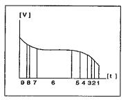
Fig. 14-3 Discharge curve for a NiCd battery This diagram shows the relationship between the battery-charge indicator and the battery output voltage.
