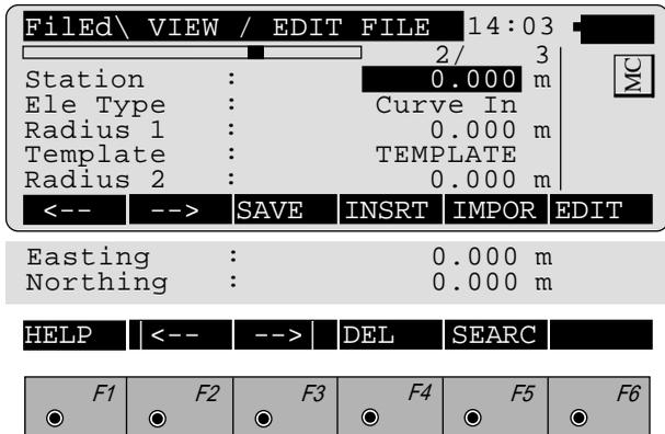
**2/ 3** : Sequence number of current point and total number of points in the measurement set. The scroll bar shows the sequential position of the measurements, graphically.
