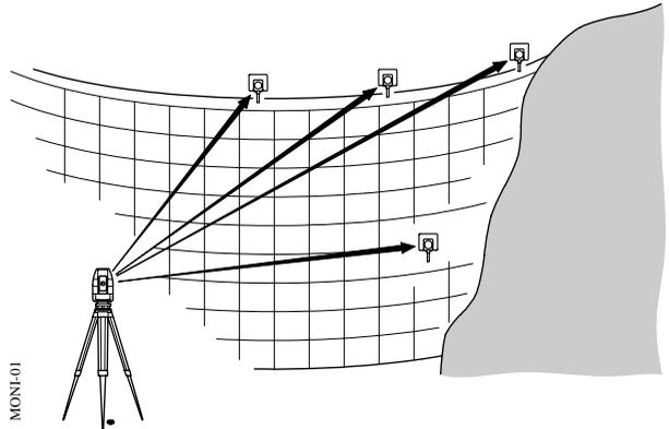
*Max. 50 measuring points and as many measurement repetitions as desired, at any time intervals.*
