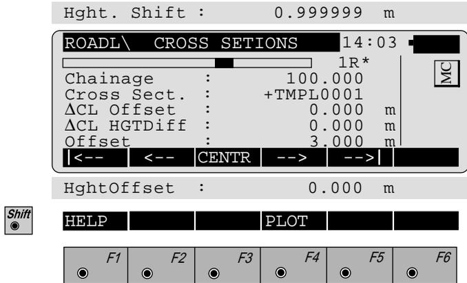
**1R** : Numbering the profile points from the centre line outwards: 1L, 2L, 3L, etc. for points to the left; 1R, 2R, 3R etc. for points to the right. The centre of the cross-sectional profile is numbered 0C. Points already set out are marked \*. The display bar displays in graphical form the position of the point in the profile.
