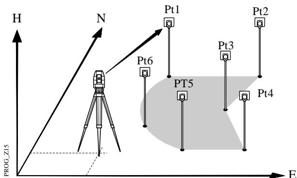
An area can be defined by a series of straight lines and arcs. Arcs are defined by 3 radial points or 2 radial points and radius.
