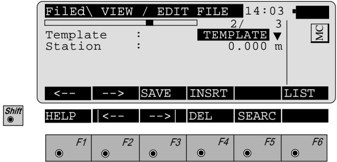
**2/ 3** : Sequence number of current point and total number of points in the measurement set. The scroll bar shows the sequential position of the measurements, graphically.
