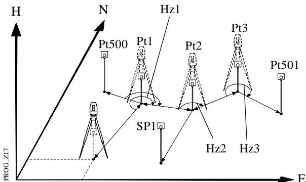
Using data about direction and distance, the program continuously computes the coordinates of the station (in the example shown above, the instrument "moves" from one station to the next, previously measured point) and aligns the horizontal circle.
