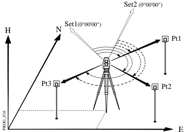
The program permits direction measurements to targets of which coordinates are not necessarily known. The average direction of all sets, the standard deviation for one observed direction and the standard deviation for the average of all directions is computed for each target. To calculate a result, a minimum of two full sets must be observed. Measurements in two faces must exist for each target .
