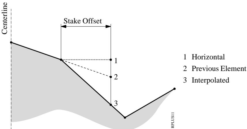
The most common method used is the "HORIZONTAL" method.
