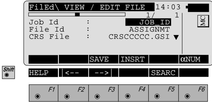
**1/ 1** : Sequence number of current point and total number of points in the measurement set. The scroll bar shows the sequential position of the measurements, graphically.
