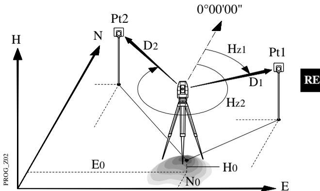
The program can be used to deduce the three-dimensional coordinates for the instrument station and the orientation of the horizontal circle from measurements to 2 target points with known Easting and Northing. To compute the position coordinates, at least the distances and the directions for both points are necessary.
