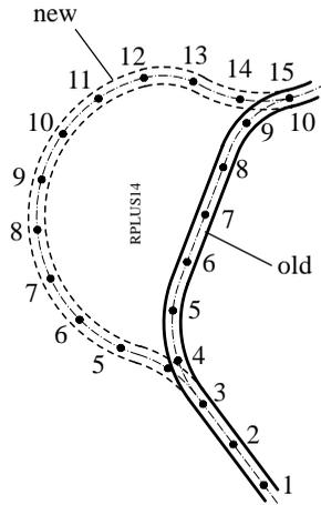
Station equations are used to adjust the alignment stationing. The most common reason for doing so is the insertion or removal of curves. Inserting or removing a curve would require re-calculating the stationing of an entire alignment. Using station equations eliminates this.
