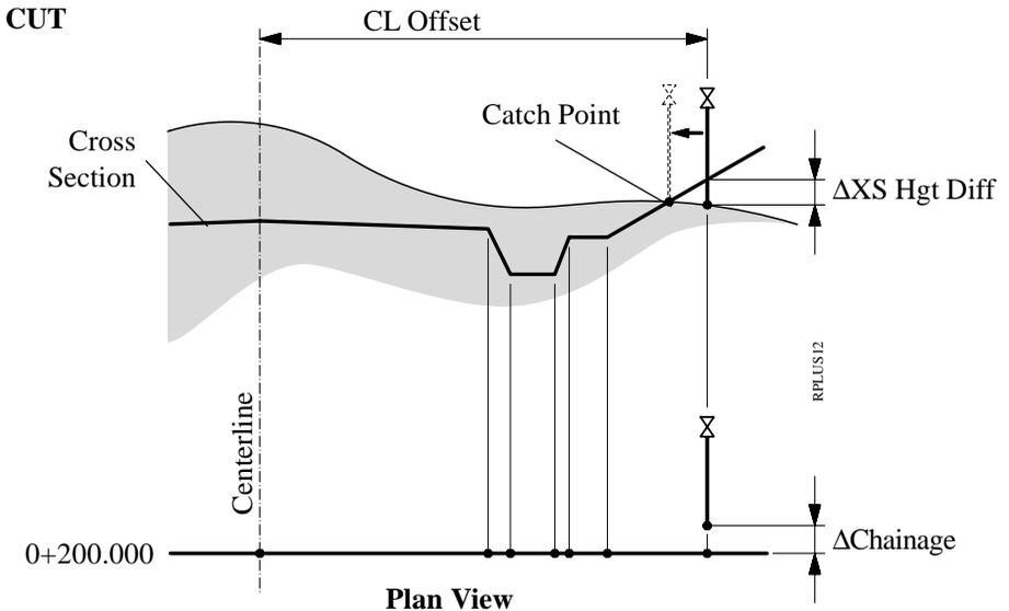
The slope staking routine is accessed from the "CROSS SECTIONS" display.
