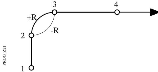
If the wrong sign (-R) is used, the arc is mirrored between the main points 2 and 3.
