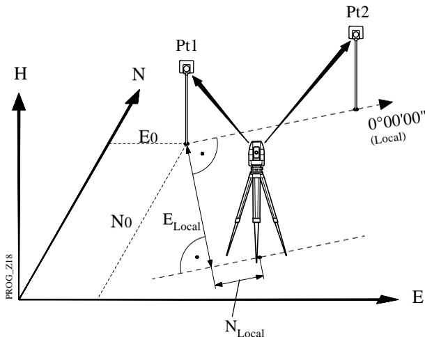
Two points are measured from any instrument station. The first point measured forms the centre of a local coordinate system ( $N=0$ ;  $E=0$ ;  $H=0$ ). The second point measured determines the direction of the positive N - axis.
