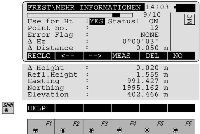
**9/10** : Sequence number of the current point and total number of points in the measurement set. The scroll bar shows the sequential position of the measurements, graphically.
