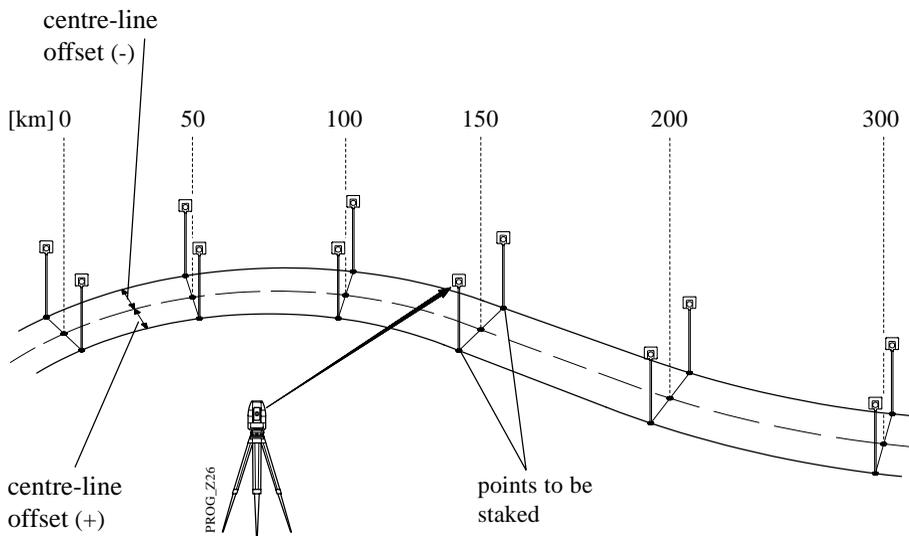
The program is suitable for setting out points which are determined by chainage and centre-line offset along a calculated alignment. If V-alignments and cross-sections are defined for the alignment, the points can be calculated and set out spatially ("ROAD STAKEOUT").
