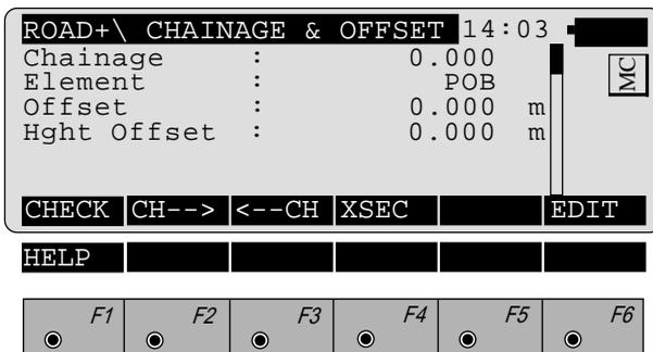
To select the template point to stake (back of curb, edge of pavement etc.):
