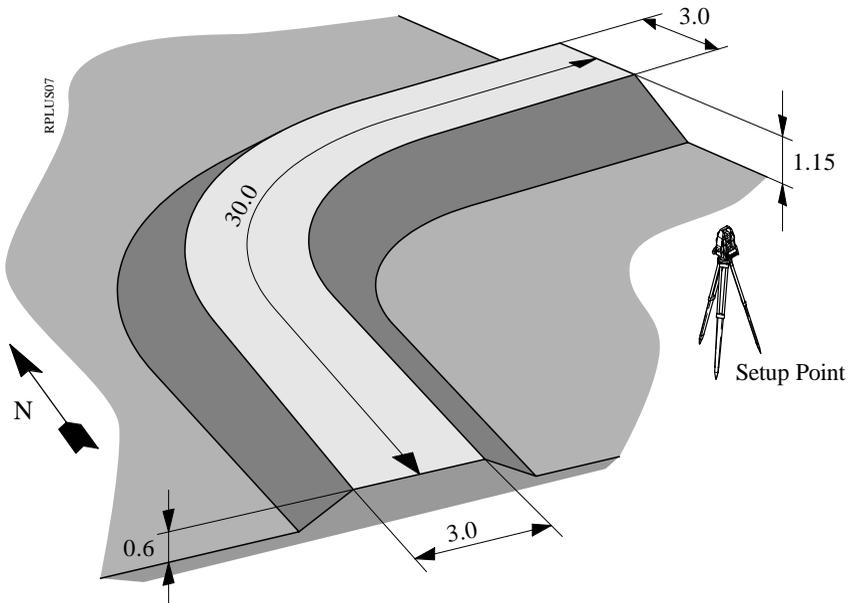
Our bike path is about 30 m in length as illustrated here. The riding surface is 3 m wide, lying 1.5 m on each side of the centerline. From the edge of the driving surface, fill slopes extend downward at a slope of 2:1.
