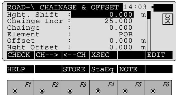
**Hght. Shift** : Vertical shift applied to the whole alignment.
