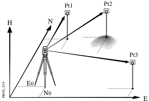
This program can be used to deduce the three-dimensional coordinates for the instrument station and the horizontal orientation of the from measurements to a maximum of 10 target points.
