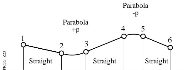
of the geometrical elements. The starting point of one element is also the finishing point of the previous element.
